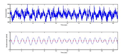
**Fig. 4.** The raw accelerometer data (top) for left-right motion is quite noisy. We can accurately and reliably detect footsteps (red circles in the bottom figure) as zero-crossings of the first derivative of the signal convolved with a Gaussian.
