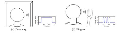
**Fig. 3.** The proximity sensor worn over the ear detects both a) when the user passes through a narrow space such as a doorway and b) when the user waves any number of fingers past the sensor. The two cases are reliably distinguished by the durations of spikes in the respective signals.
