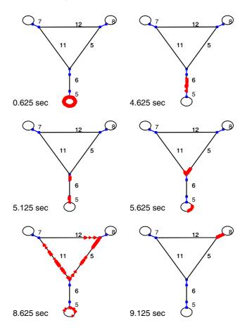
**Fig. 6.** Tracking results. As the subject passes through three doorways in succession, the motion model propagates particles along edges according to detected footsteps, and each particle is weighted by comparing observed and expected sensor readings.
